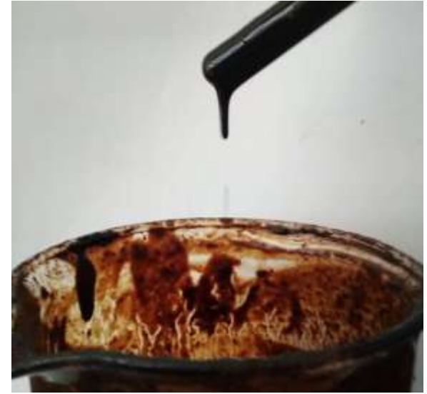
Total liquefaction of Sludge after PARALAX® treatment
